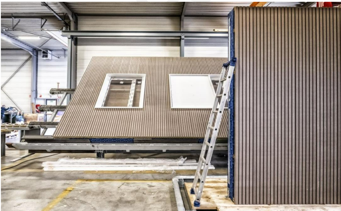
Figure 33. Final steps of the production of prefabricated wall elements, by BuildUp Offsite Construction Company, https://www.buildupoffsite.com/nl_BE/blog/buildup-nieuws-1/how-does-offsite-construction-contribute-to-meeting-the-un-sustainable-development-goals-14 . Copyright by BuildUp.
